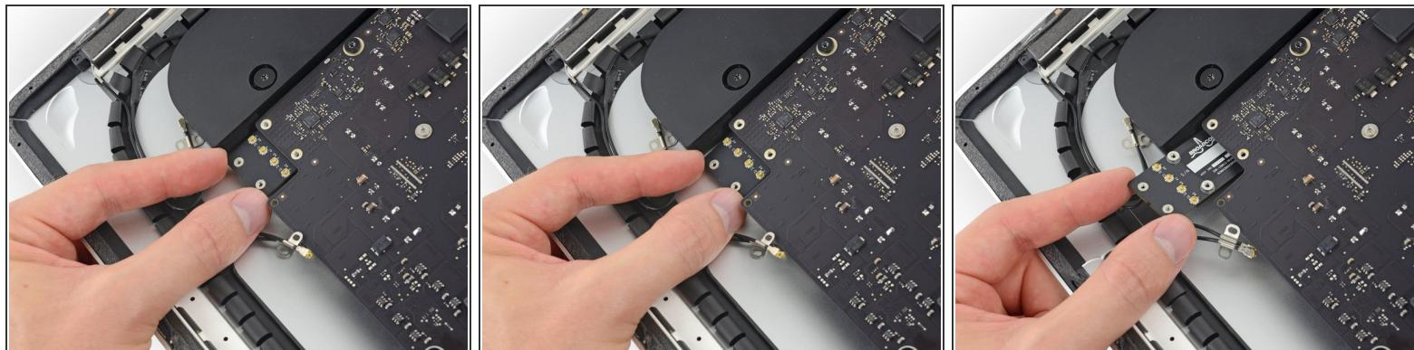
⚠ Do not push the AirPort/Bluetooth card away from the logic board more than 1-2 mm. Doing so may cause severe damage.
